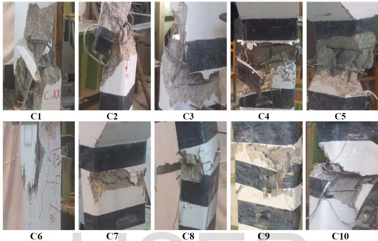
Figure (2): Failure modes of the tested samples
